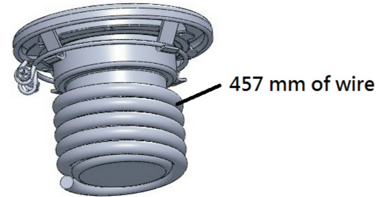
Figure 2 Cord to coil around the back of the light fixture
